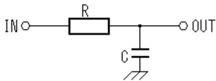
$$\begin{aligned} V_{out}/V_{in} &= 1/(j*\omega*C) / (R + 1/(j*\omega*C)) \\ &= 1/ (j*\omega*C*R + 1) \end{aligned}$$
